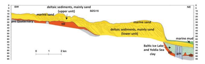
Fig. 3. Geological cross-section of submerged part of Vistula Delta (acc. to seismoacoustic data)
