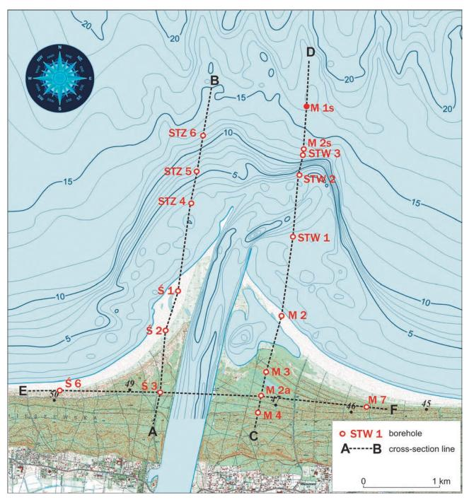
Fig. 11. Drilling sites and cross section lines
