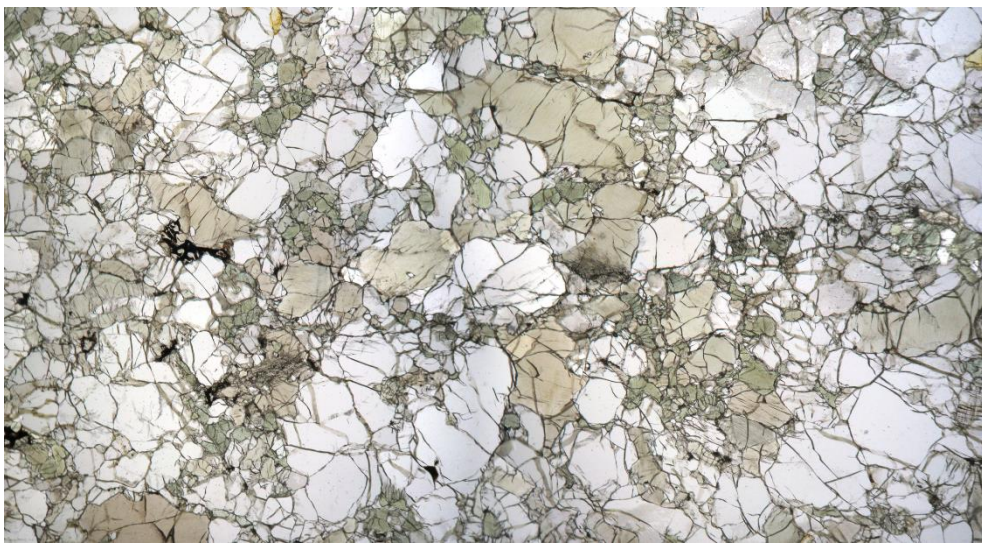
Peridotite from Montboissier quarry, Massif Central, France. Optical image, plane polarized light. Width of the photo ~4 cm. (photo: J. Puziewicz & M. Matusiak-Małek)
