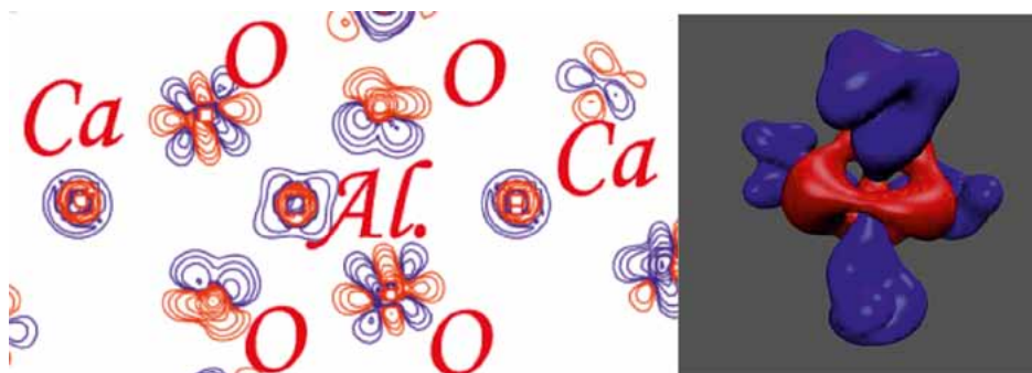
Fig. 1. (left) Redistribution of electron density at O and Al ions under high pressure, and (right) the 3D SiO 4 deformation electron density maps at ambient conditions – isosurfaces: blue colour +0.1 e/A 3 , red colour -0.1e/A 3 .
