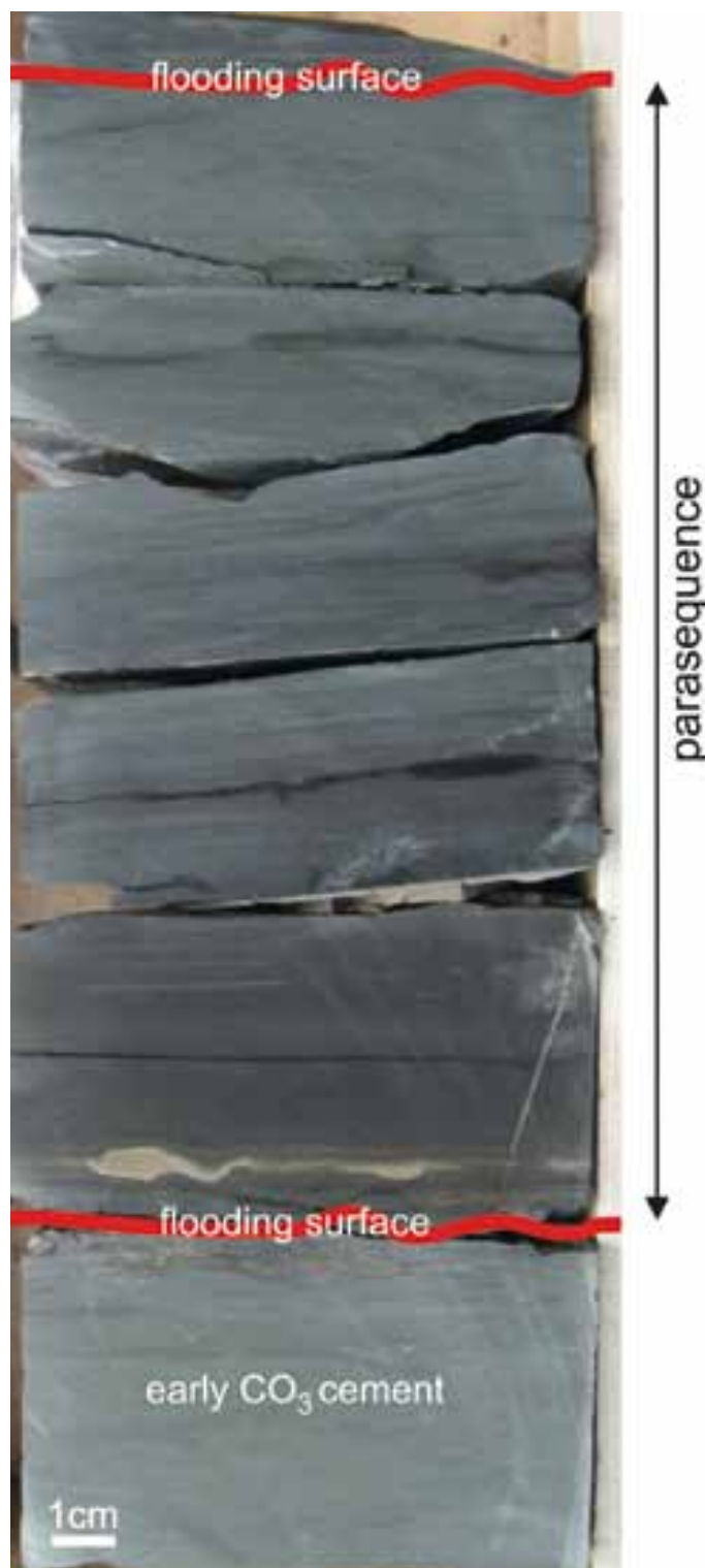
Fig. 17. Part of drillcore displaying flooding surface and interval with early carbonate cementation. Most parasequences are thicker than this one, used for illustration
