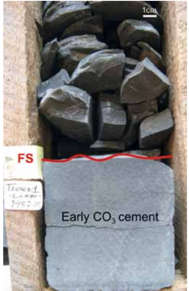
Fig. 12. Early carbonate cementation in Tłuszcz IG-1 well; FS – flooding surface
